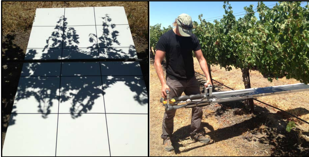
Figure 1. Crop coefficient ( K_c ) was determined by measuring shaded area under trellis at solar noon with a grid board, 50 days after bud break (left) and Paso Panel, 100 days after bud break (right). K_c values were 0.34 and 0.24 at 50 days after bud break and 0.34 and .31 at 100 days after bud break for sites 'A' and 'B' respectively.
